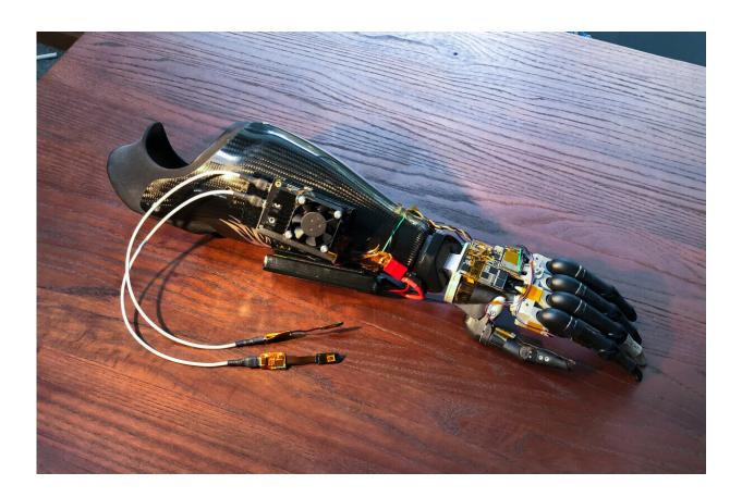
When combined with an artificial intelligence computer and the above robotic arm, the University of Minnesota researchers' neural chip can read and interpret brain signals, allowing upper limb amputees to control the arm using only their thoughts. Credit: Neuroelectronics Lab, University of Minnesota
