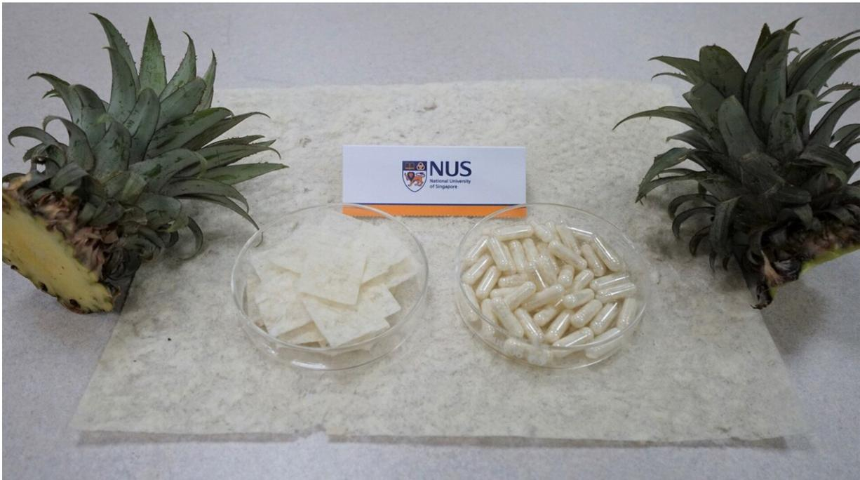
Upcycling agricultural waste such as pineapple leaves for high-value applications such as fat absorption can help reduce waste and increase profits of farmers. Similar fat-trappers can also be made using other types of cellulose fibres such as sugarcane bagasse and coffee grounds. Credit: National University of Singapore
