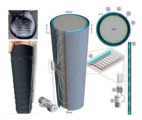
Images of the lymphedema sleeve (left) and a diagram of its components (right). The microfluidic chip sequentially inflates and deflates balloons, creating pressure and pushing fluid through the arm. Credit: Carolyn Ren
