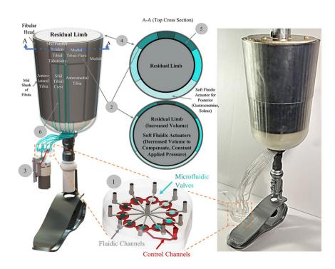
Proof-of-concept rendering (left) and photo (right) of the prototype of the new microfluidics-enabled soft robotic prosthesis for lower limb amputees. Credit: Waterloo Microfluidics Laboratory at University of Waterloo
