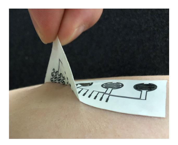
Photograph showing the stickiness between the wearable concept and human skin. Credit: Missouri University of Science and Technology
