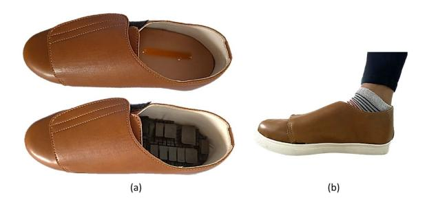
(a) Footwear with self-offloading insole underneath the top sole (b) one of the volunteers wearing the self-offloading footwear. Credit: Priyabrata Maharana, Jyoti Sonawane
