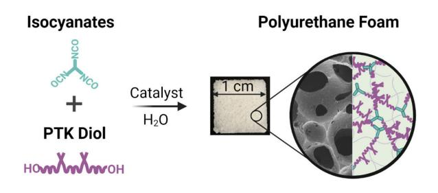
A schematic illustrating the design and interior structure of the polyurethane foam, which forms pores that allow for cell infiltration. Credit: P. Patil, et al.
