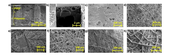
(a) full thickness cross-section of PVDF400 and (b) PVDF-only layer crosssection. Surface of (c) PVDF layer and (d) polyester support layer. SEM images of N95 layers (e) 1, (f) 2, (g) 3, and (h) 4. In mask orientation, layer 1 is exposed to the open environment and layer 4 is exposed to the inside of the mask. Layer 3 is referred to as the "separating" layer, as it had the highest flow resistance. Credit: University of Kentucky
