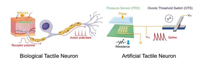
Schematic diagram comparing the components of biological tactile neurons and artificial tactile neuron devices developed in the research. Credit: Korea Institute of Science and Technology (KIST)
