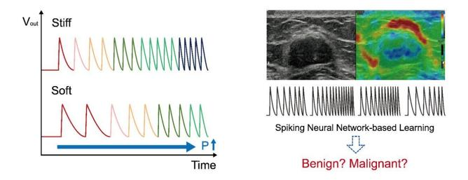
(left) Spike evolution pattern examples of the artificial tactile neuron device according to the stiffness of the pressed material, (right) Example of determining whether a tumor is malignant or benign by AI learning of ultrasound elastography images of a breast tumor using the stiffness-encoded spike patterns. Red indicates soft areas, and blue indicates stiff regions. Credit: Korea Institute of Science and Technology (KIST)
