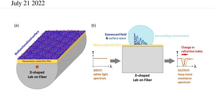
a) 3D view of the nanofunctionalized D-shaped lab-on-fiber sensor. b) Related sensing mechanism based on the evaluation of refractive index changes, through evanescent wave interaction, that occur in the fiber surface and are determined by the spectral shift of the LMR, which is generated by a metal-oxide thin film. Credit: *Advanced Photonics Research* (2022). DOI: 10.1002/adpr.202200044
