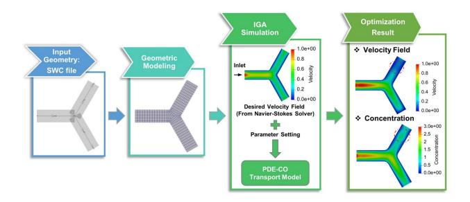
An overview of the material transport control simulation in a bifurcation geometry. The traffic jam is introduced by reducing MTs in the red dashed circle region. Color bars unit for velocity field: μμm/s and concentration: mol/μμm22. Credit: Angran Li and Y.J. Zhang, *Scientific Reports* (2022). DOI: 10.1038/s41598-022-07861-6
