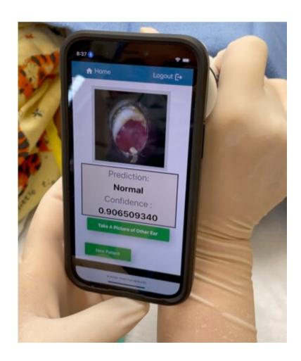
OtoDx is currently being employed in a prototype device paired with a smartphone app. The device acts as a "mini otoscope" that would fit over the phone's camera and allow clinicians to take photos of the inside of a child's ear, upload them directly to the app and receive a diagnostic reading in seconds. Credit: Mass Eye and Ear
