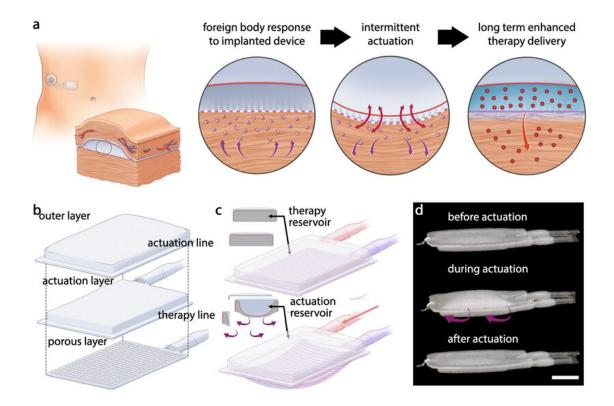
The drug-delivery system includes an actuator that repeatedly inflates and deflates the device for five minutes every 12 hours. This mechanical deflection prevents immune cells from accumulating around the device. Credit: William Whyte et al
