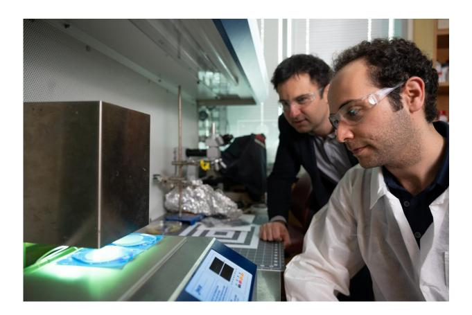
Fabrication of the microchip. The device is fabricated by injecting a polymer into a micro fabricated mold and the polymer is cured under ultraviolet light to produce low-cost, single-use devices. Credit: Georgia Institute of Technology
