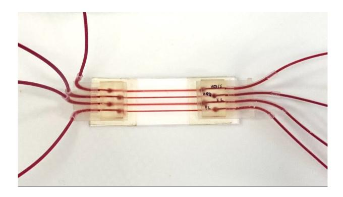
The tiny tool closely replicates short sections of human blood vessels, allowing researchers to create variable flow conditions which are very close to those found in the body. Credit: McMaster University
