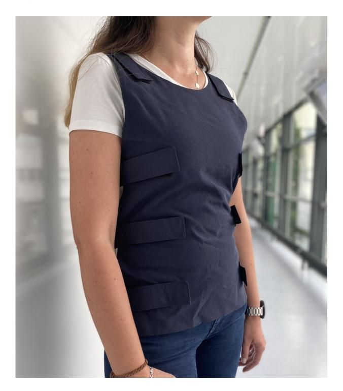
Acoustic sensors are integrated into the front and back of the textile vest to listen to the thorax. Credit: Fraunhofer-Gesellschaft
