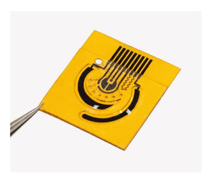
A version of the sweat sensor. The large curved sections are electrodes that stimulate sweat production. Credit: Caltech
