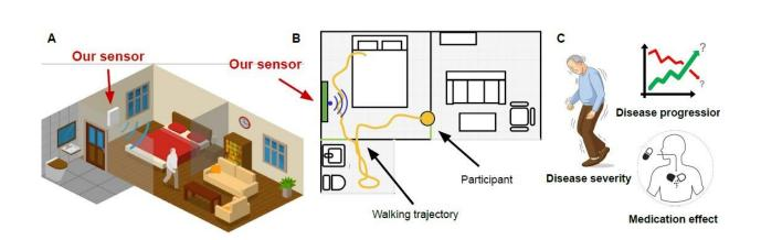
The sensor operates like a low-power radar, where it captures radio waves to assess patients' walking patterns, their disease progression, and the effects of medications. Credit: Liu et al., *Sci. Transl. Med.* 14, eadc9669 (2022)
