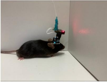
The study involved the use of biosensors, algorithms and open-source software to build a miniature microscope. The findings contribute to a better understanding of how our brains track and retain information about routes and learn new locations (miniature microscope recording electrical activity of neurons in mice. Credit: Archive of Peter J. Schuette et al
