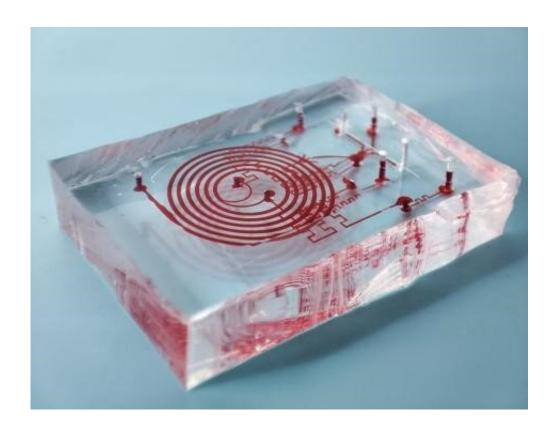
Scientists from Hangzhou Dianzi University proposed a 3D-stacked multi-stage inertial microfluidic sorting chip for high-throughput enrichment of Circulating Tumor Cells (CTCs) and convenient downstream analysis. Credit: X. Xu, Hangzhou Dianzi University
