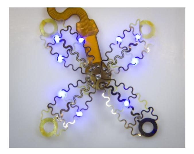
The device uses light and a technique called optogenetics, which modifies cells that are sensitive to light, then uses light to affect the behavior of those cells. Credit: Philipp Gutruff
