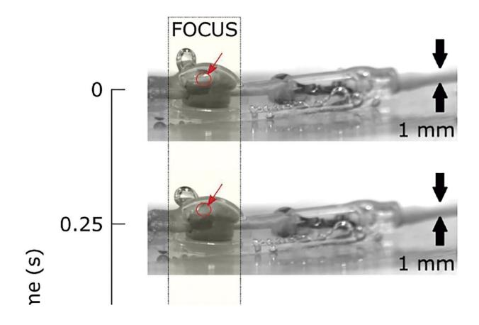
Selection of photograms from demo video (Video 2) demonstrating cavitation inside a hydrocephalus valve filled with water and graphite powder over. The graphite tracer at t=0 is deposited on the lower wall of the valve in the absence of ultrasonic waves. The remaining photograms illustrate resuspension of the graphite particles within 1 second of ultrasonic radiation. Credit: Universidad de Sevilla
