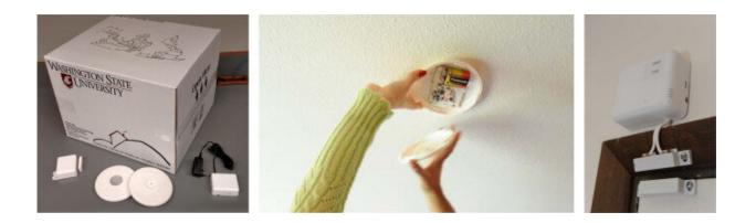
(left) The CASAS Smart Home in a Box (SHiB) contains (middle) passive infrared (PIR) motion detectors coupled with ambient light sensors and (right) magnetic door use detectors coupled with ambient temperature sensors. When there is a change in state, sensors indicate the new state in a text message sent to a central Raspberry Pi. This machine tags the message with the corresponding date, time, and sensor identifier. Credit: *Pain Management Nursing* (2022). DOI: 10.1016/j.pmn.2022.08.011
