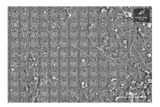
Scanning Electron Microscope image of a neural culture that has been growing for more than six months on a high-density multi-electrode array. A few neural cells grow around the periphery and have developed complicated networks which cover the electrodes in the center. Credit: credit Cortical Labs
