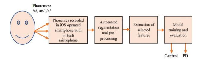
The block diagram of identifying PD from HC using sustained phonemes. The model is trained and tested using 72 PD and HC participants. Credit: *IEEE Access* (2022). DOI: 10.1109/ACCESS.2022.3203973
