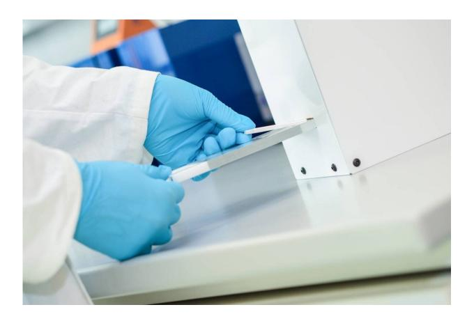
Test chip, in which the proband sample is applied and a light reaction determines the result. The chip consists of a cartridge and a microstructured polymer film. Credit: Fraunhofer-Gesellschaft
