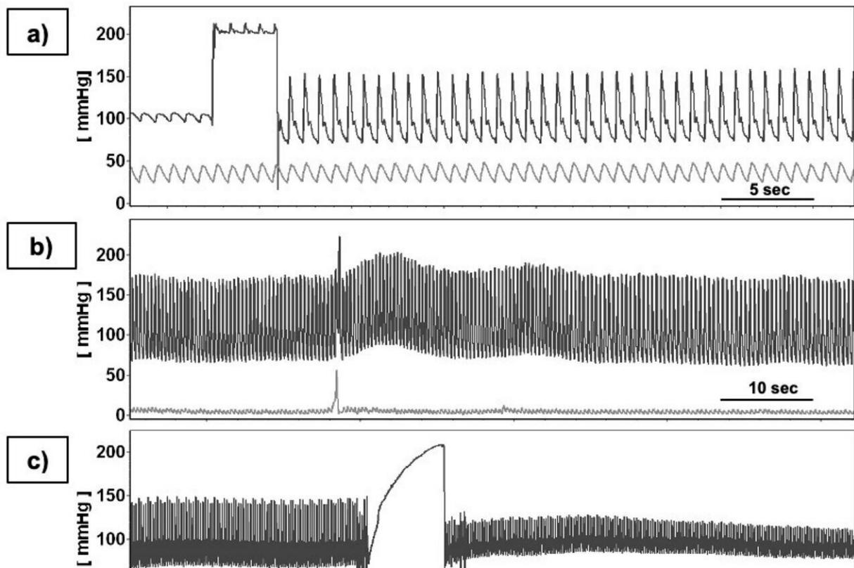
Effect of artifacts upon the pressure reactivity index. Identified shapes of artifacts: (a) rectangular, (b) fast impulse, (c) saw tooth, (d) isoline drift, (e) constant value.
