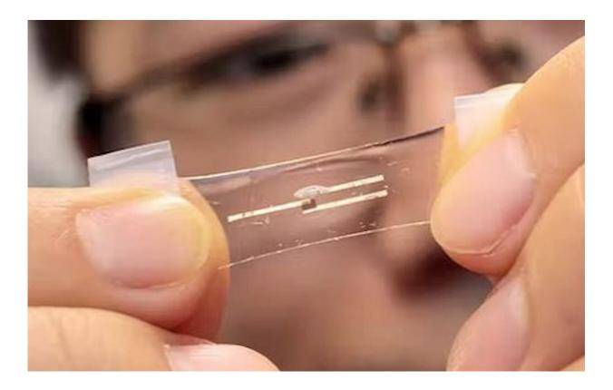
These electronic circuits are flexible and stretchable. Credit: UChicago Pritzker Molecular Engineering/John Zich, <u>CC BY-ND</u>
