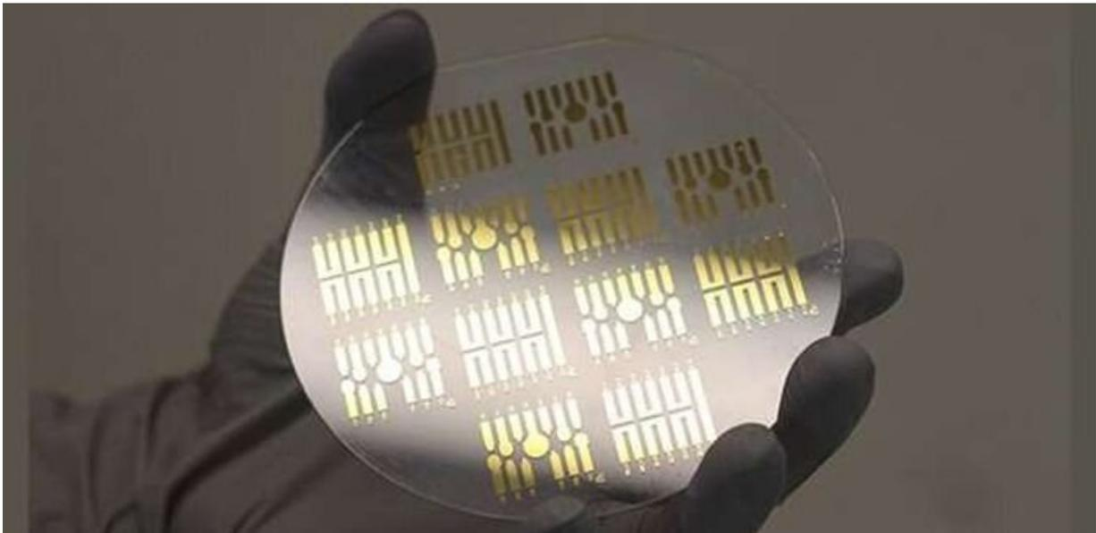
Scalable thin film transistor-based biosensors. Credit: Ben Woodington, University of Cambridge
