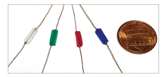
Examples of MAGENTA prototypes fabricated with a "shape memory alloy" spring and an elastomer, and how their sizes compare to that of a one cent coin. Credit: Wyss Institute at Harvard University
