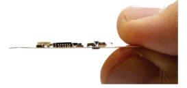
Photographs of the smart bandage showing the microcontroller unit (MCU), crystal oscillator, high-pass filter (HPF), stimulation and sensing electrodes, flexibility of the printed circuit board, adhesion of the hydrogel interface to skin, and thin layout of the board. Credit: Jian-Cheng Lai, Bao Research Group @ Stanford University
