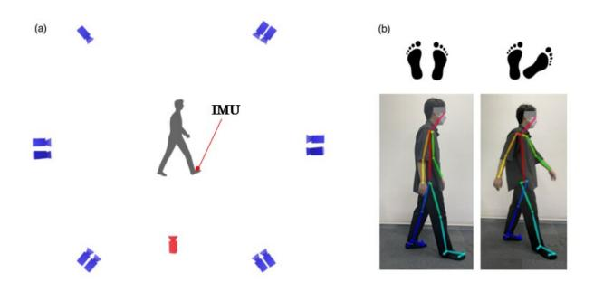
TUS researchers develop a method that enables accurate gait analysis by combining information from a small inertial measurement unit (IMU) attached to the shoe with estimated information on the bones and joints of the lower limbs, obtained by capturing the gait from a single RGB camera. Credit: Masataka Yamamoto from Tokyo University of Science.
