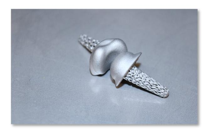
The FingerKIt implants are produced using special 3D printing processes which enable a high level of detail and different surface qualities. Credit: Fraunhofer IAPT
