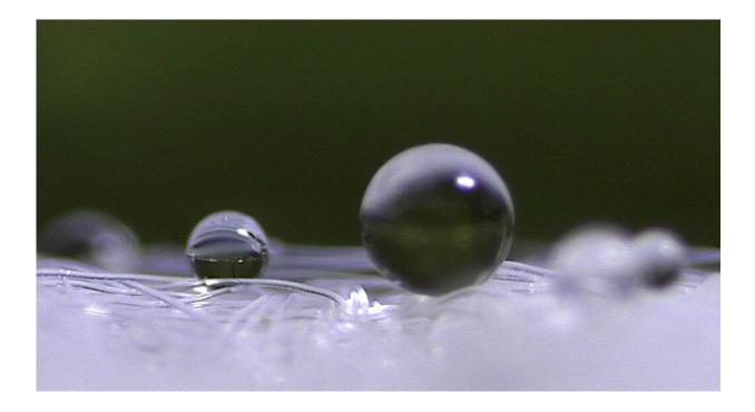
An optical image showing the large water droplets (1-5 mm in diameter) deposited on the microfibers of an N95 type mask. Credit: Sang Jin Park et al
