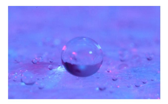
An optical image showing the water droplets in various sizes (0.2-5 mm in diameter) deposited on the fibrous surface of an N95 type mask. Credit: Sang Jin Park et al.
