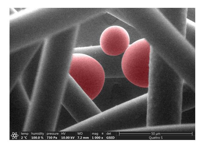
An SEM image showing the smaller water droplets (5-20 micrometers in diameter) deposited on the microfibers of an N95 type mask. Credit: Sang Jin Park et al
