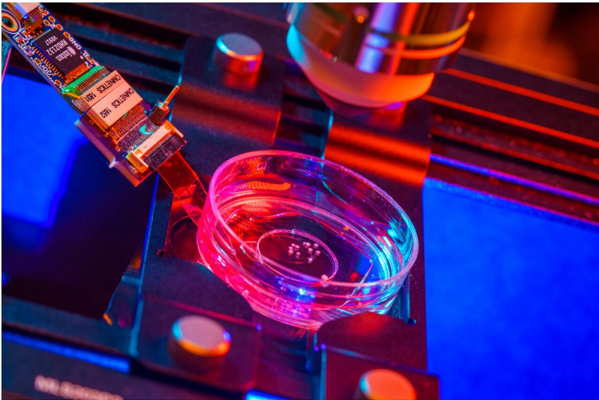
The researchers developed experiments that combine microelectrode arrays made from transparent graphene, and two-photon imaging, a microscopy technique that can image living tissue up to one millimeter in thickness. Credit: David Baillot/UC San Diego
