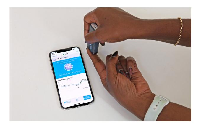
The malaria detection tool collects an infrared signature for a mobile phone to process. Credit: The University of Queensland
