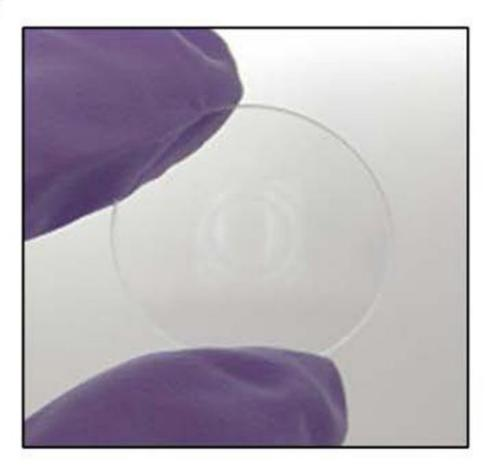
A diffractive optical element (DOE) used in NB-PAM. Credit: Caltech
