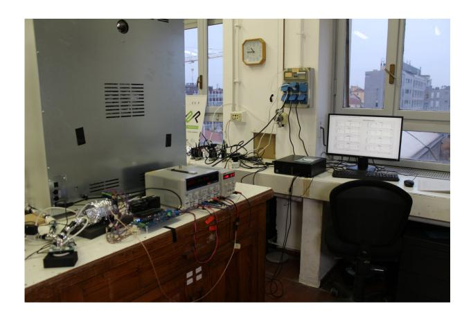
Prototype of an electronic nose developed by the Politecnico di Milano in partnership with Humanitas, capable of diagnosing a tumor using a urine sample with 82% accuracy. Credit: Politecnico di Milano
