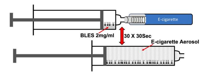
Schematic of the in vitro surfactant exposure set-up. Aerosol exposed surfactant was generated using a syringe containing BLES connected directly to an EC device which allowed aerosol to be drawn into the syringe and, after 30 seconds, expelled. This procedure was repeated 30 times. Credit: *PLOS ONE* (2022). DOI: 10.1371/journal.pone.0272475
