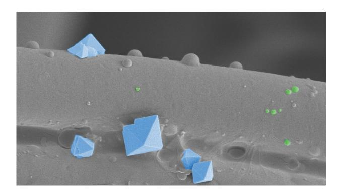
Only a few viruses make it to the innermost layer of a fabric mask. The picture shows a textile fiber with salt crystals (light blue) and viruses about 100 nanometers in size (green). (Scanning electron microscopy, colored) Credit: Empa
