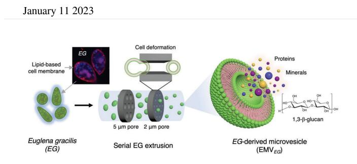
Schematic illustration for fabrication of EMVEG using a EG extrusion method. Credit: *Advanced Materials Interfaces* (2023). DOI: 10.1002/admi.202202255
