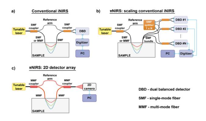
A schematic diagram of conventional interferometric near-infrared spectroscopy (iNIRS, a) is compared to two possible implementations of parallel iNIRS ( $\pi$ NIRS, b, c). Credit: *Biomedical Optics Express* (2022). DOI: 10.1364/BOE.472643
