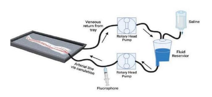
Perfusion of an amputated limb with saline and a fluorescent agent (i.e., fluorophore) administered via a dominant artery. The saline and targeted fluorophore entered via the artery, the limb was drained through gravity, and the perfusate recycled back into the circuit. Credit: *Journal of Biomedical Optics* (2023). DOI: 10.1117/1.JBO.28.8.082802
