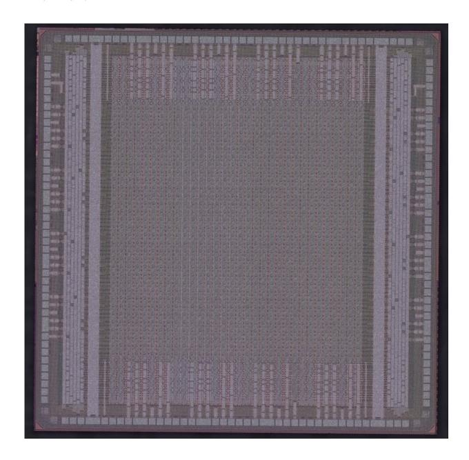
A close-up view of the custom readout integrated circuit. Credit: Lincoln Laboratory research team
