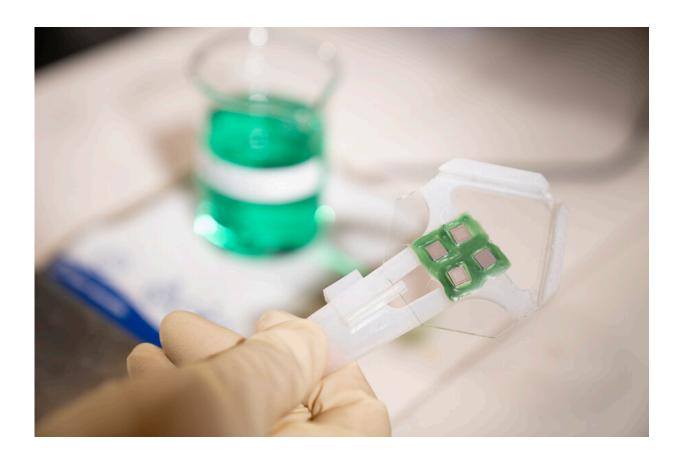
Four custom readout integrated circuits are mounted so that they can be placed on metal plating. The Geiger-mode avalanche photodiodes are layered onto this circuit and they work together to capture and record the photon signals. Credit: Glen Cooper
