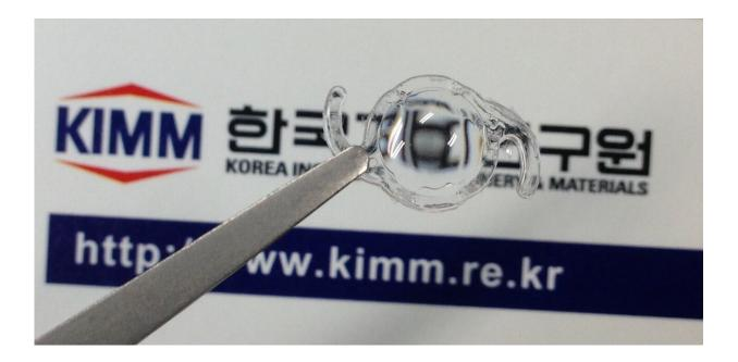
Lens used in the development of smart intraocular lenses. Credit: Korea Institute of Machinery and Materials (KIMM)
