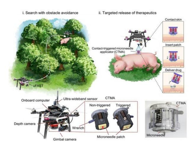
Figure 1. Schematic and physical diagram of the UAV autonomous drug delivery system for first aid. Credit: *Advanced Materials* (2022). DOI: 10.1002/adma.202208648
