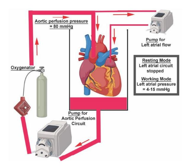
A graphic depicting the set up for the ex-vivo pig heart infusion apparatus.
