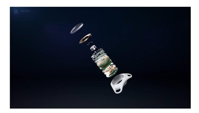
Complex functionality in a tiny capsule: The microimplant consists of an eight-layer circuit board. Credit: WILDDESIGN GmbH, Gelsenkirchen
