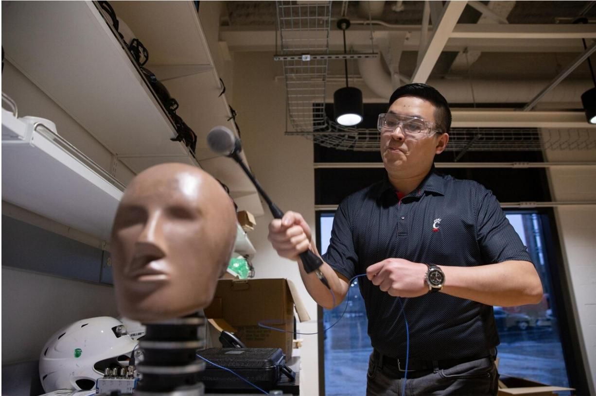
UC Biomedical engineering student Shengming Hu uses a modal hammer to strike a dummy head containing accelerometers. By comparing the force the dummy registers with and without a helmet, researchers can see which helmets provide better protection from potential concussions. Credit: Andrew Higley
