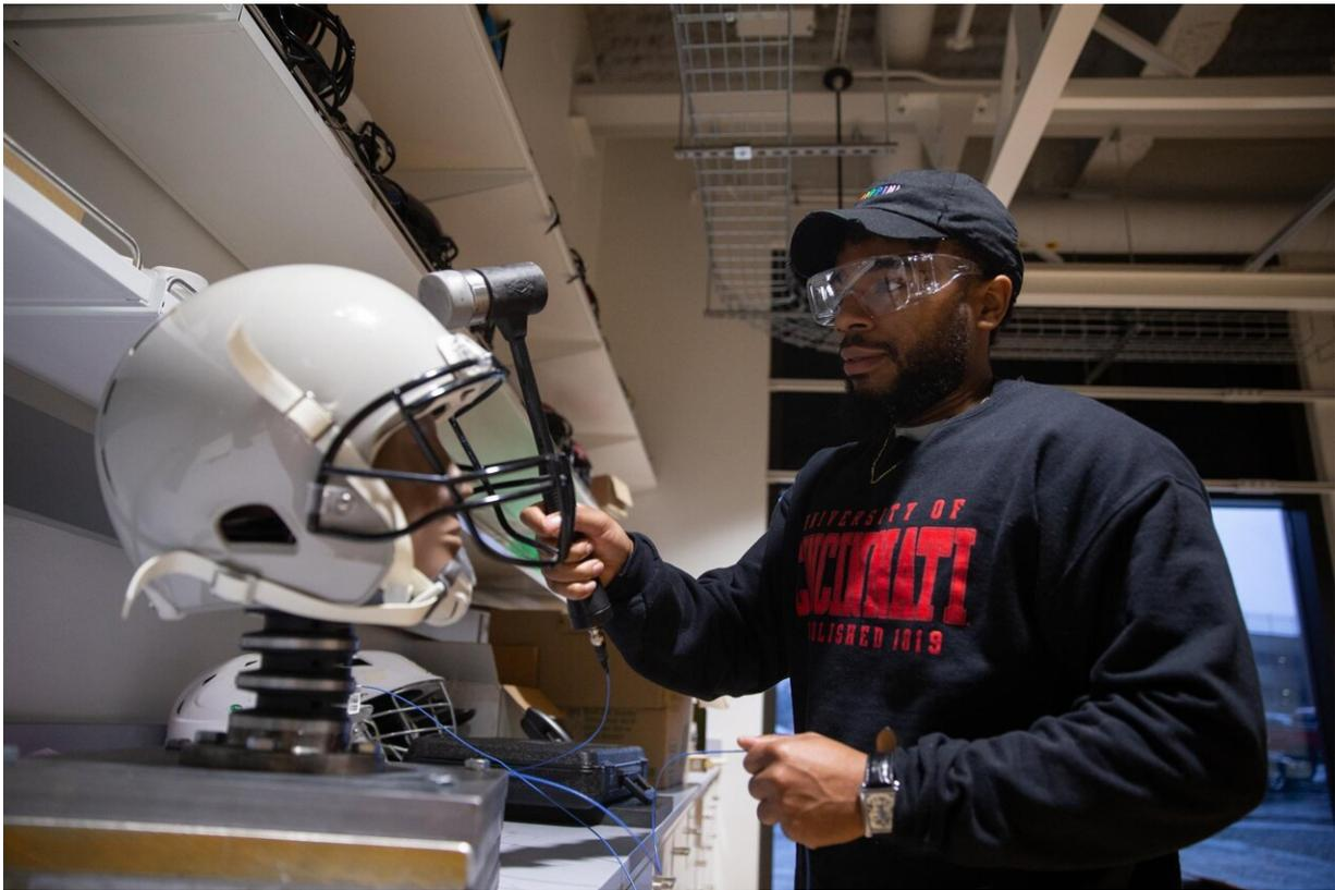
UC Biomedical engineering student Christopher Boles uses a modal hammer to strike a dummy head containing accelerometers. By comparing the force the dummy registers with and without a helmet, researchers can see which helmets provide better protection from potential concussions. Credit: Andrew Higley
