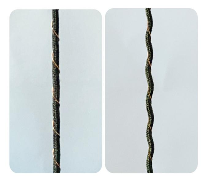
Garn: A rigid wire (orange) is wrapped in spirals around a length of elastic rubber (black)—both are conductive. Left slack, right stretched. Credit: Tyler Cuthbert / ETH Zurich
