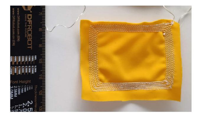
The antenna is sewn directly onto the material in loops. Credit: Valeria Galli / ETH Zurich
